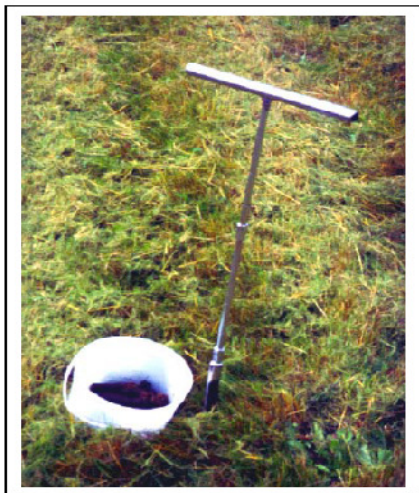
Figure 2 Soil Sampling Equipment
